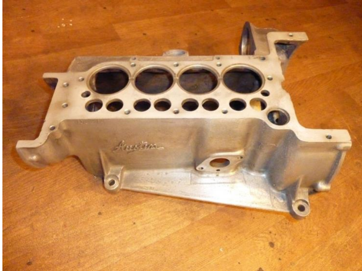
Carefully lapped flat top surface
