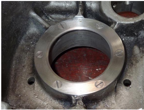
Replacement ring in position
