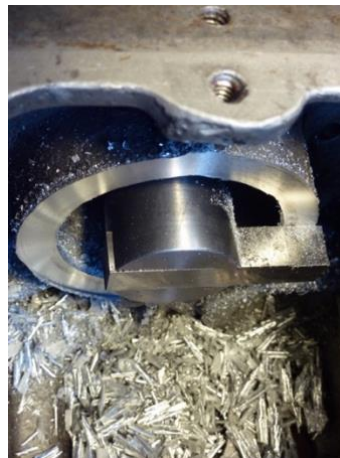
Flange being removed
