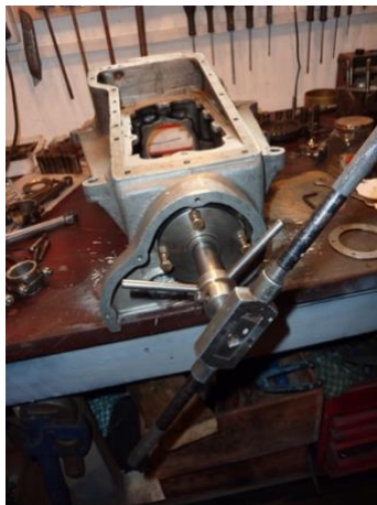
Flange removal tool
