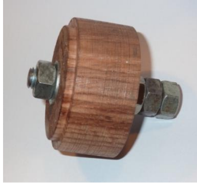
Jig to ensure ring is concentric
