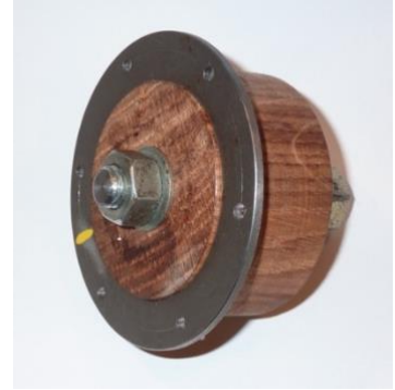
Ring in position on jig
