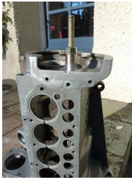
Extractor in position
